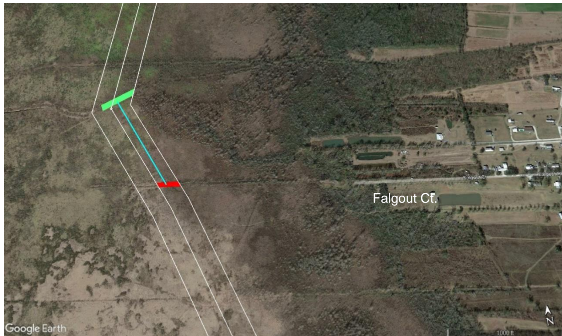
Figure 42. New canal (blue) to direct water from dead-end canal (red) to canal with water control structure (green)
